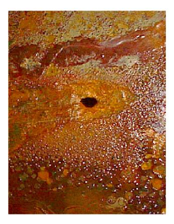
In these areas it is recommended to check the plate thickness on a regular basis to avoid such problems and to renew the plate in good time to prevent holes occuring.
