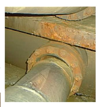
It is recommended therefore, that ship's personnel should pay particular attention to these pipes when inspecting ballast spaces in the normal course of planned maintenance and cleaning, and that any damaged securing hoops should be replaced as soon as possible.
