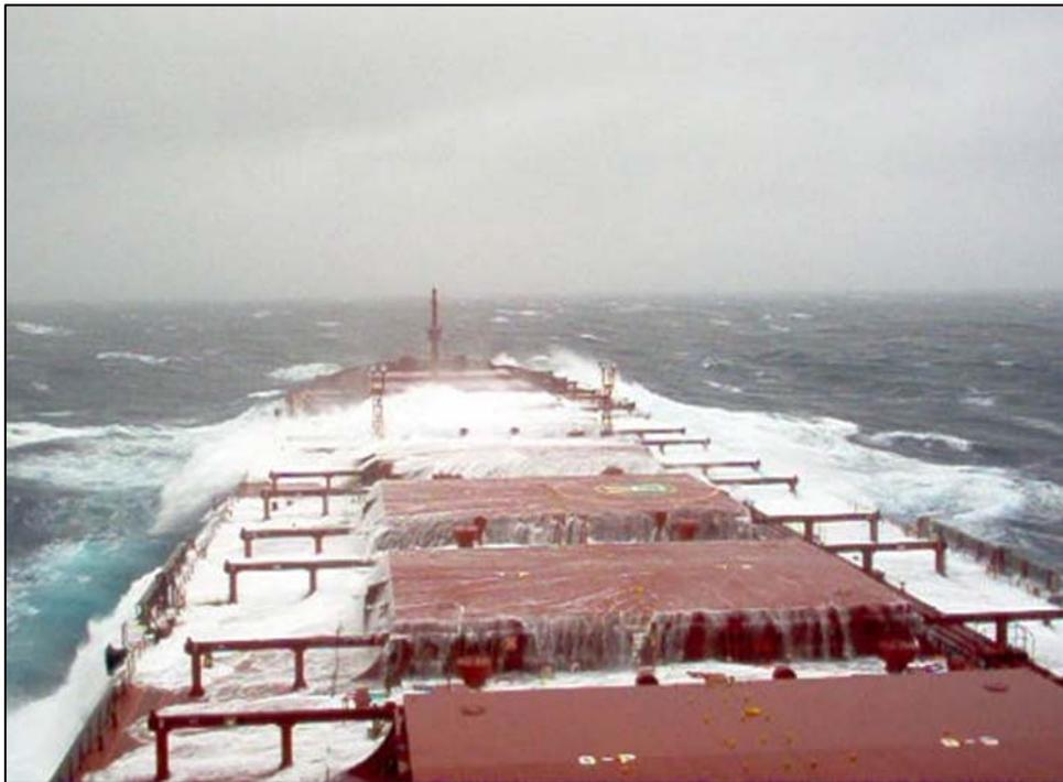
If the work is considered essential, weather forecasts and the prevailing sea conditions should be continuously monitored so that ample warning may be given to enable ships staff to secure the vessel and move to a safe area before the adverse or heavy weather is encountered. Accidents have occurred when crew members have ventured out on deck to secure items that were not adequately secured, either prior to sailing or when the vessel was in sheltered waters.
