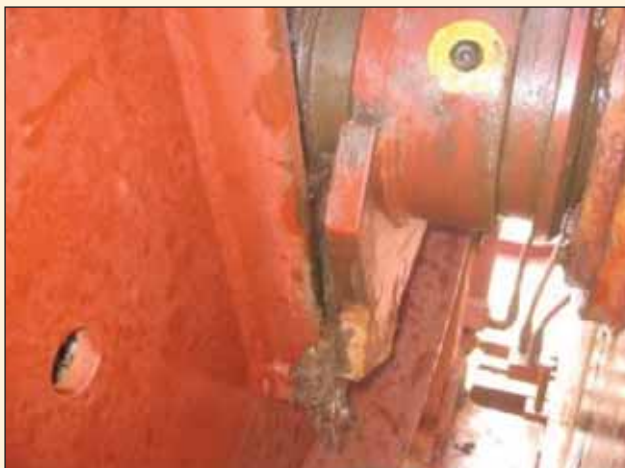
▲ View of dog clutch into which the parka sleeve and hand were drawn
