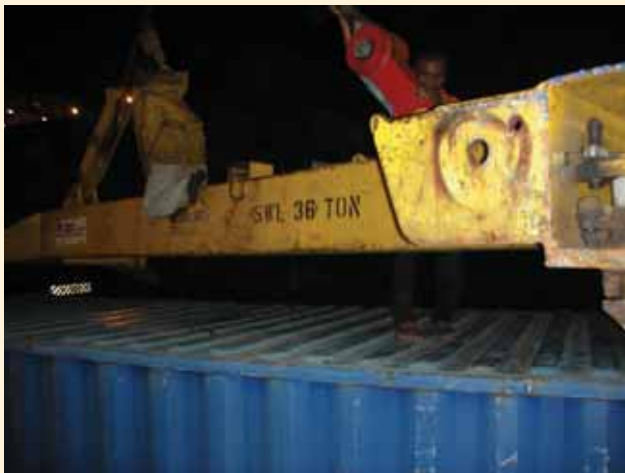
▲ 1: Manhandling the spreader: one worker has no shoes and the other is wearing 'flip-flops'
