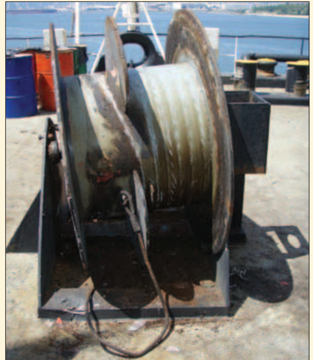
▲ 1: View of damaged towing wire drum showing broken end fittings. The centrifugal brake system is housed within the reel.
