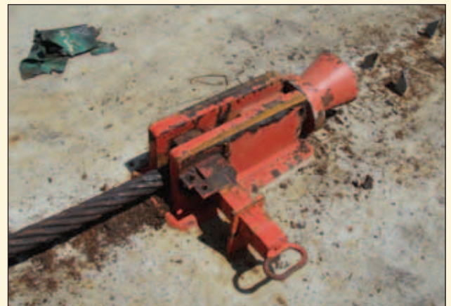
▲ 2: Heavy end of towing wire successfully held by strong point.
