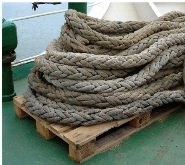
**Ropes correctly stowed off deck**
