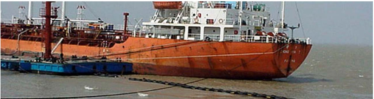
The ship has correctly put out as many lines as possible but should also consider the use of the anchor and mooring lines running aft from either the main deck or other suitable areas. In situations like this it is important to analyse local tidal and weather patterns in order to predict how the vessel will be affected. The vessel owners should be informed and cargo operations stopped (or not commenced) if conditions do not appear safe.
