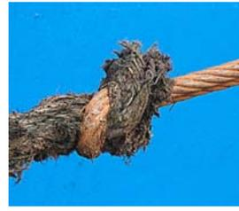
A rope mooring line should never join a metal line without the use of a thimble.
