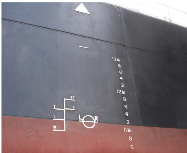
An example of the load line or 'Plimsoll' mark painted on the side of merchant ship
