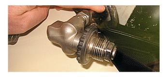
It is not uncommon to see that this valve has been secured to the apparatus using spanners or other hand tools. This should not be done, tightening by spanner
