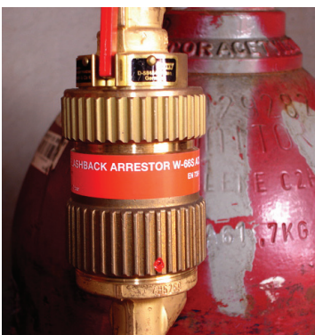
Flashback arrestor fitted
