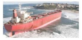
she was approaching the beach. Inevitably the vessel grounded with both anchors in their hawse pipes.
