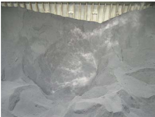
Signs of heating in a coal cargo
