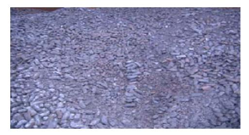
The attached photograph shows the degree of breakage of the briquettes in this case and in particular the vast quantity of fines present. The fines offer an increased surface area exposed to oxidation and reaction with any water or moisture present in the hold atmosphere. In a marine environment any water or moisture would have a salt content which would accelerate the rate of oxidation and hydrogen evolved.
