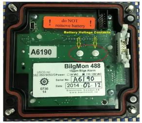
circumstances should the battery be removed. Furthermore, a red warning sticker is affixed to the circuit board as pictured above. Attempting to remove the battery in this circumstance may cause an unrecoverable error, failure and data loss. A manufacturer's representative indicated that the battery was originally designed to last the lifetime of the device and that if the RTC stops due to a power supply
