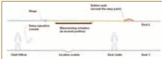
▲ Figure 1: Arrangement of hinged internal ramp
