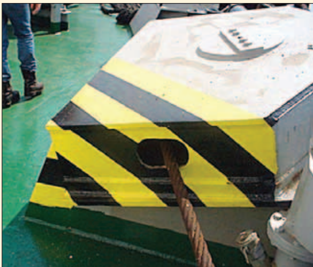
▲ Figure 1: Obstruction / trip hazard highlighted with 'tiger' stripes
