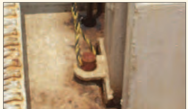
▲ Figure 1: View of modified eyepad and securing pin to secure lifeboat davit
