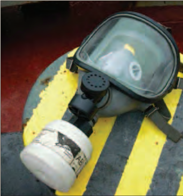
▲ Figure 7: 'Heavy duty' dust mask which the cadet could have mistaken for an EEBD. Such masks should be clearly marked 'Not for use in oxygen-deficient atmosphere' in a language understood by the crew.
