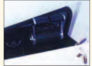
▲ Figure 4: Bridge wing control station being folded into storage recess. Due to limited size of the opening, the engine control levers have to be moved down to full ahead position for storage.
