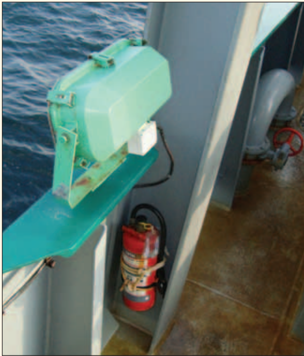
▲ Figure 7: Inappropriate location (main deck bulwark on a low-freeboard ship) for a portable fire extinguisher. This can result in: i) the extinguisher getting damaged or washed overboard by shipped seas, and ii) corrosion gradually weakening the body and increasing the risk of it rupturing under pressure when used in emergency or training.
