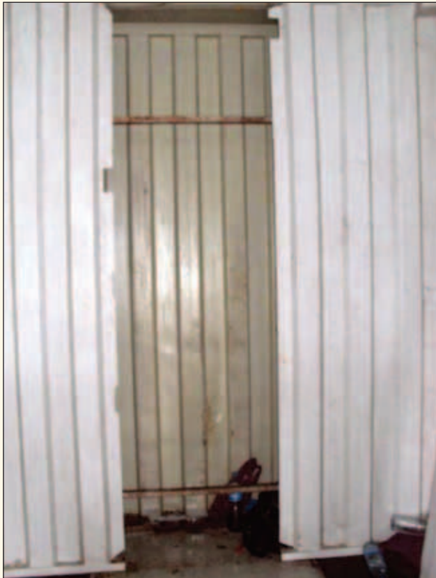
▲ Figure 6: Closer view of the false end panel, showing the space that hid 10 stowaways during inspection on shore by ship's crew
