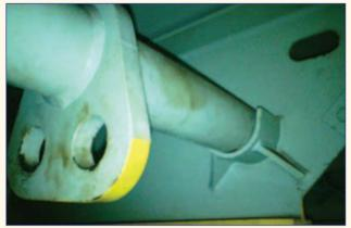
▲ Figure 3: Close up view of portable pipe 'spreader' with lugs. Note that the end supports have no securing arrangements to prevent the inadvertent dislocation of the portable spreader
