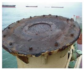
The main cause of the crane failure is still unclear. However, it was established that considerable time had elapsed since the stores crane was last tested / inspected. The ship had left drydock two weeks previously where the ship's main derricks had been tested and the Cargo Gear Book revalidated but no testing / inspection of the stores crane had taken place.
