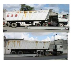
We are advised that instead of uncoupling the trailer the front end of the unit is weighed, the unit then drives through leaving the rear axle on and another reading taken. The readings are then added together. This is done both empty and full the difference being the weight of the commodity.
