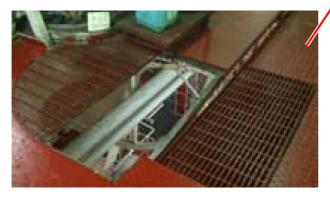
The grating of an opening on the 3<sup>rd</sup> deck level in the engine room of the entered vessel was removed so that a ladder could be passed through it. Unfortunately a young crew member was unaware of the unguarded opening in the deck and fell through it and later died due to his injuries. The image (right) indicates the height of the fall.
