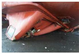
water at which point it was checked and confirmed that the hooks were holding. Unfortunately, as the lifeboat was then being recovered it suddenly fell from a height of five metres, causing the death of a crew member inside and serious injury to others.
