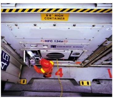
electrician should perform any repairs that are necessary for the refrigerated container. The electrician should have access to a set of different reefer manuals for all the various types and manufacturers of reefer containers laden onboard the vessel. In addition, a basic set of spare parts for the various types of reefer containers should be kept onboard to effect necessary repairs. system should be in place that allows for continuous access and replenishment
