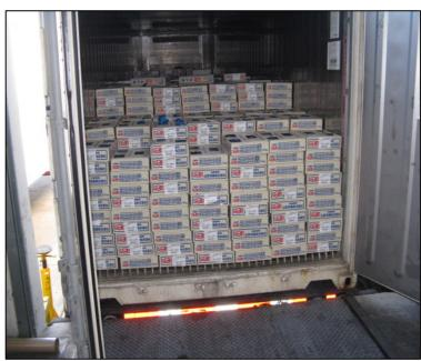
The terminal personnel should document, in part, the refrigerated container number, the temperature and vent setting, the weight of the container, cargo and chassis and the seal number on the equipment interchange receipt ("EIR").
