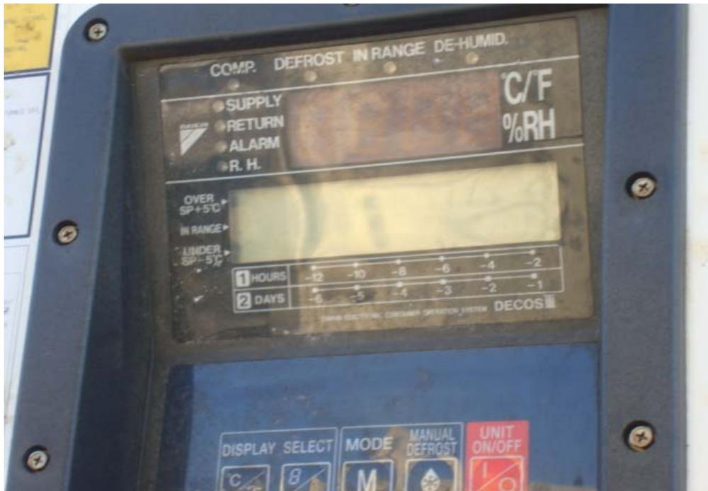
The above photo is a reefer container control panel, which is where the reefer technician inputs the shipper specified thermostat setting for the carriage of the perishable cargo. The vessel and yard checker record the temperatures from these screens on the monitoring logs.
