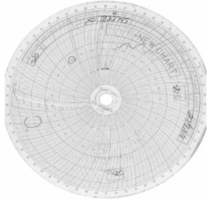
The above chart covers a shipment, which was booked to be carried at -20°C. Although the chart only covers a few days, you can see that the baseline temperature when the refrigeration unit was not in defrost mode was maintained at the required temperature. Note the large defrost spikes are
