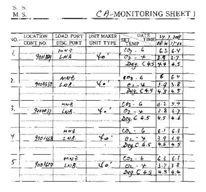
In the above log, the vessel's reefer engineer recorded the container number, the load and discharge ports, the unit size, and the CO2 set point; the O2 set point and temperatures in "degrees C". All 3 readings are within acceptable ranges on this date.
