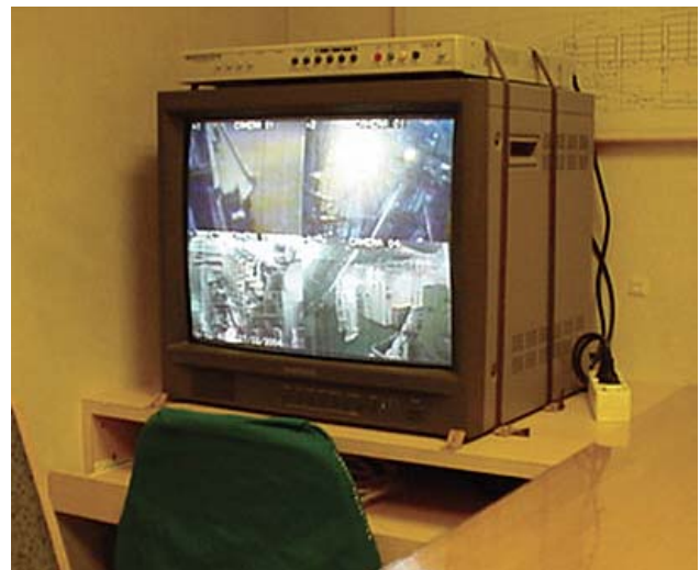
Here, it is possible to photograph all visitors to the vessel. Records are stowed on a disc or tape, and would be very useful during times of a security alert.
