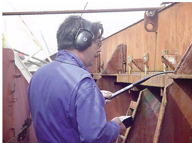
Ultrasonic testing of hatchcover
