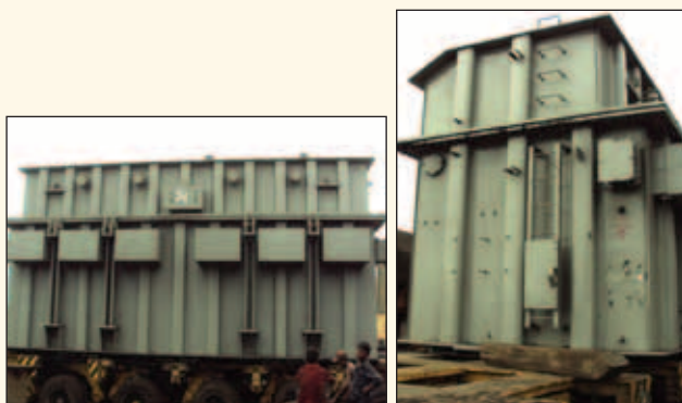
▲ Figure 1: A heavy lift without proper shipping marks
