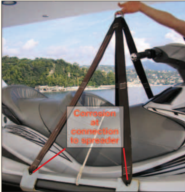
▲ Figure 3: Typical PWC slinging arrangement
