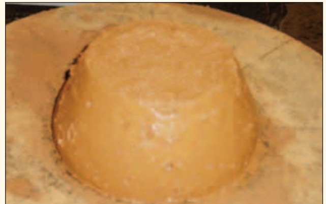
▲ Figure 2: Change in shape of sample cone after testing, corresponding to a 6.5mm cone expansion
