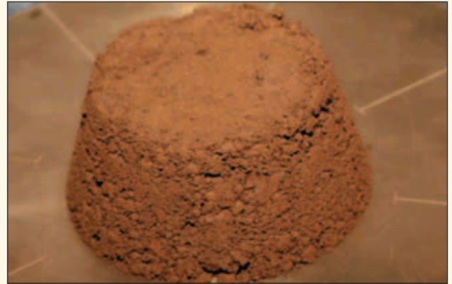
▲ Figure 1: Typical shape of sample cone prior to testing
