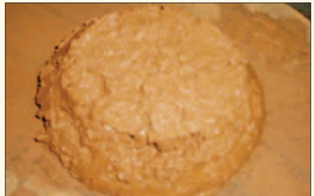
▲ Figure 3: Sample cone after testing with 20mm expansion at base
