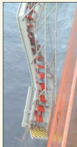
▶ Another view of damaged accommodation ladder
