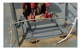
As the drugs must be carried onboard a ship the means of access to the ship should is the first concern. Areas such as the **Hawse pipe** on the fo'c'stle are often overlooked and may well have been left free and open as the anchors will have been cleared prior to port entry. The hawse pipe should be secured, as illustrated, to prevent unwanted 'visitors' to the vessel. The Spurling pipe leading to the chain locker should also be
