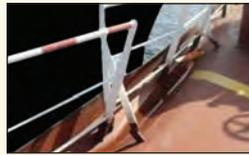
▲ Close up view of damage to sheerstrake and upper deck railings on own vessel
