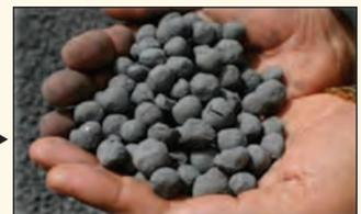
▶ Figure 2: DRI (B), Lumps, pellets, cold moulded briquettes
