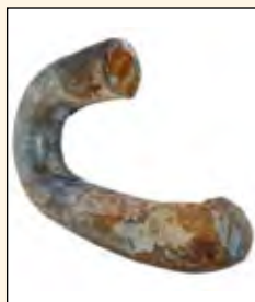
▲ Broken link of chain later recovered from deck
