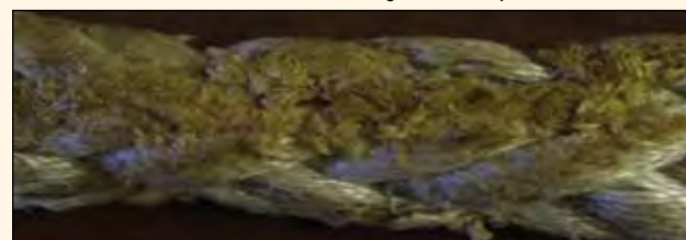
▲ Evidence of abrasion damage near the failure zone
