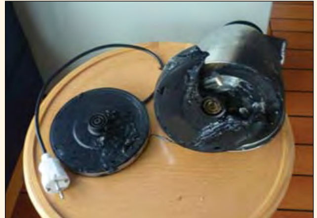
▲ View of fire-damaged kettle and base unit
