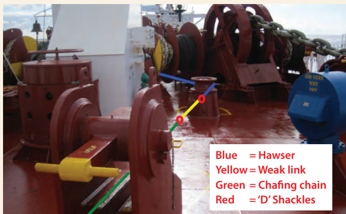
Illustration of mooring arrangement before commencing heaving on the hawser – note the sharp nip around the pedestal roller
