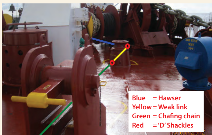
Illustration of mooring arrangement after the hawser was heaved in with the weak link sharply nipped on the pedestal roller. The pear link parted at this point.
