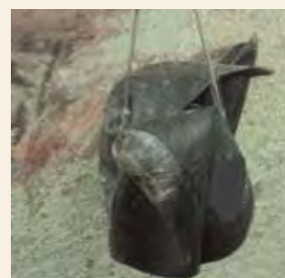
Damaged pneumatic fender hanging by wire sling and chain
