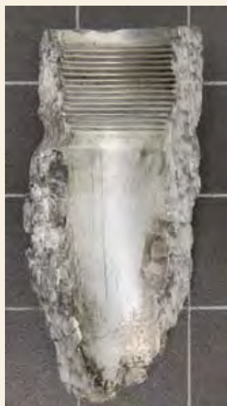
View of adaptor that allowed the dangerous connection of SCBA air compressor discharge line to OBA oxygen cylinder
