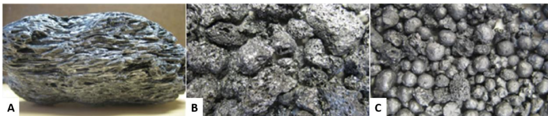
Figure 1. Some of the petcoke types. A. Needle petcoke; B. Sponge petcoke; C. Shot petcoke. Source (Edwards, 2015) 2 .
