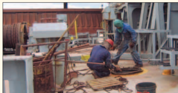
▲ Figure 4: Crew members hauling out cleaning equipment through the deck opening
