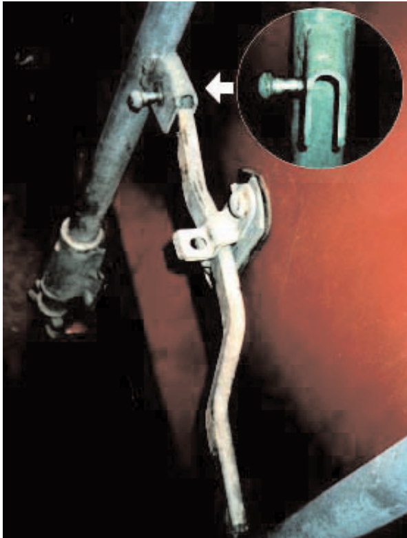
Main photo and inset show part removed pin on sealed door handle
