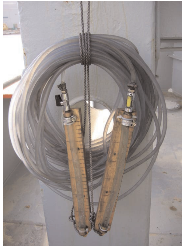
Above: Manometer showing plastic tubing (30-40 m long), fitted at each end with a valve and scale. The valves are to allow the water in the tube to be retained without any air bubbles in it when the device is not in use.
