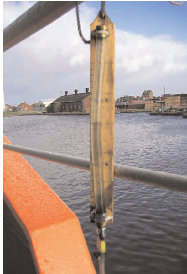
Below: Manometer, showing scale and water level. When a scale is fitted and used for the reading care must be taken that the scale is fixed at the same height on each side.
