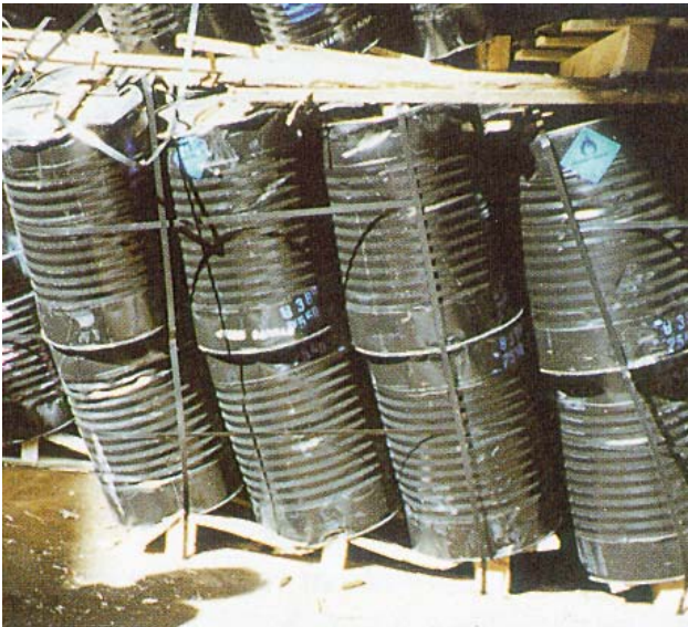
Heavy drums that have broken loose from inadequate strapping
