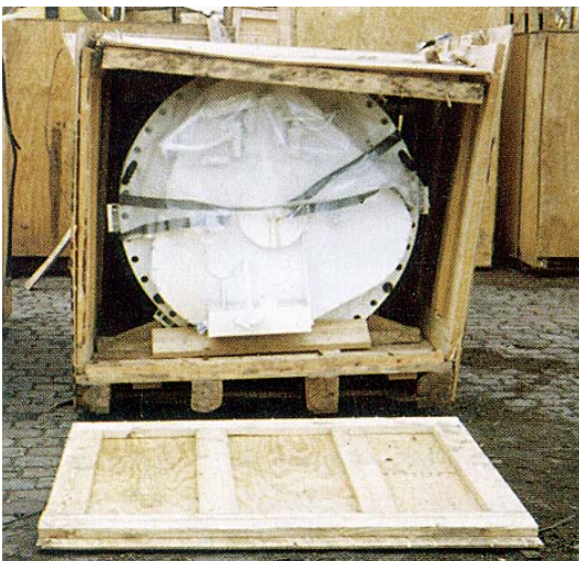
Wooden cases that lack structural rigidity
