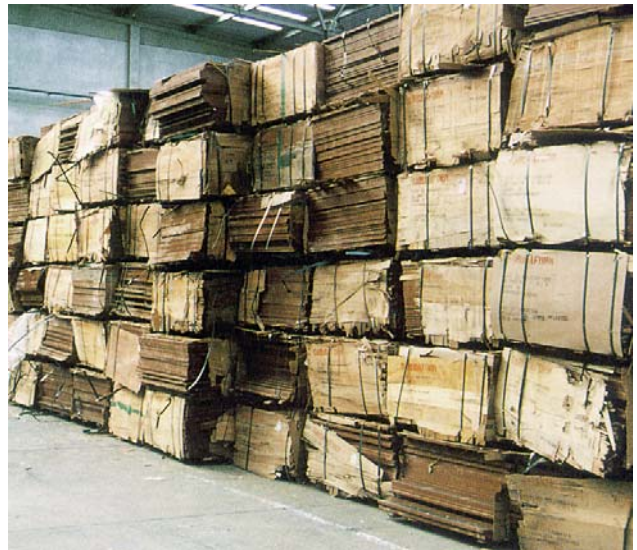
Plywood bundles that have broken out of packing that is insufficient for the weight of the bundles and bearers
