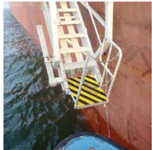
Bottom platform not horizontal
